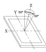
Inspection should be performed within  $\emptyset$  ( $\emptyset$ =30°) from Z axis to each X and Y axis.
