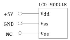
Note: There is an end on the potentiometer for regulating contrast ratio.
