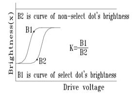
Contrast Ratio (K) =  $\frac{\text{Brightness of non-selected dot (B2)}}{\text{Brightness of selected dot (B1)}}$
