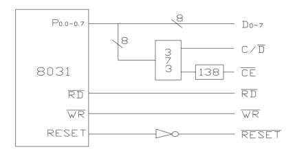
Data bus of 8031 is connected directly to the data bus of module. RD and WR of 8031 act as the read/write control signal of module. CE can be decoded by address bus. For example: output Y0 of IC 138 as CE. (When test the module independently, CE could be grounded directly.) Output A0 of 8031 address bus as C/D. A0=1 stands for the address of command; A0=0 stands for address of data. Each Subprogram is as follows:
