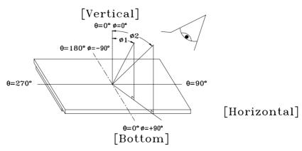
Note: <4>Definition of viewing angle  $(\Delta \Phi) \Delta \Phi = |\Phi - \Phi 2|$
